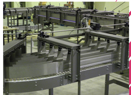
This guide rail system features a hand-wheel and digital counter that provides adjustment of all the lanes from one side of the conveyor system.
