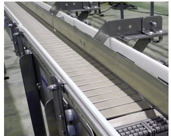
This hinged rail provides off-center product travel and flips out of the way when not required.
