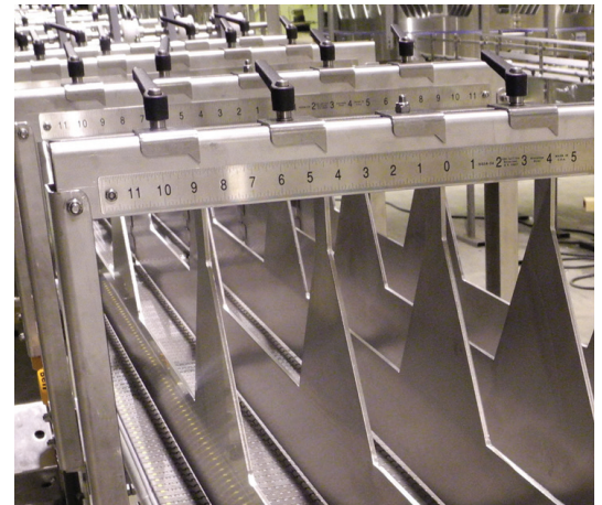
This change-over system, utilizing a ratchet handle and a bolt-on ruler guide, alleviates measuring on manual guide rail adjustments.
