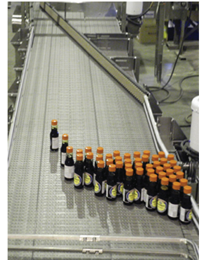
Due to the low back pressure benefits, the Pressure-less Combiner is often used to single file glass bottles to reduce breakage.
