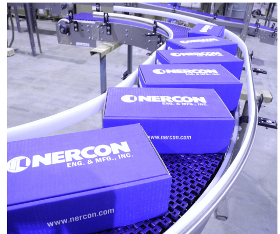
Products must be controlled through turns to prevent skewing.
