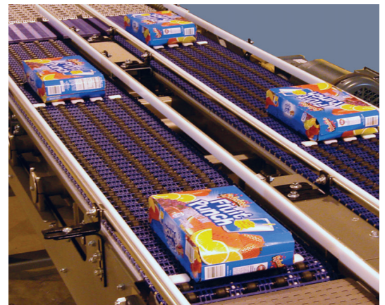
The Live Roller Metering/Merging conveyor system shown here is handling over-wrapped products.
