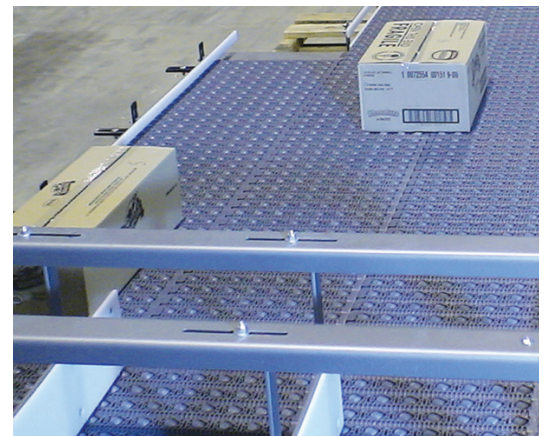
This ARB system utilizes a Vision system that scans the bar codes and sends the signal to control the direction of cases into specific lines.
